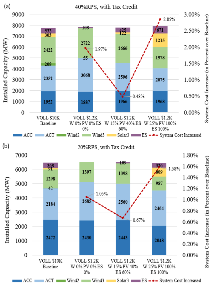
Fig. 3. Resource mixes and increases in system cost relative to Baseline Model EO resulting from EC model with low, medium, and high arbitrary CCs under different levels of RPS (a. 40 % and b. 20%) (Note: marginal CCs under Model EO under 40% RPS: Wind2, 22%; Wind3, 1.5%; Solar3, 48%; ES 82%; under 20% RPS: Wind2, 32%; Wind3, 1.6%; Solar3, 67%; and ES 100%)
